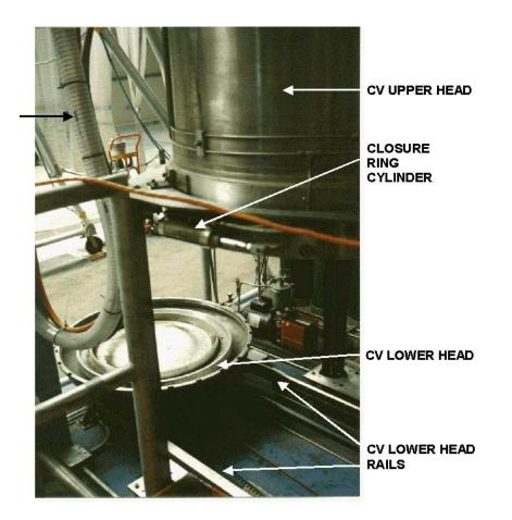
Figure 1-9. Drum Venting System Ready for Drum Loading
