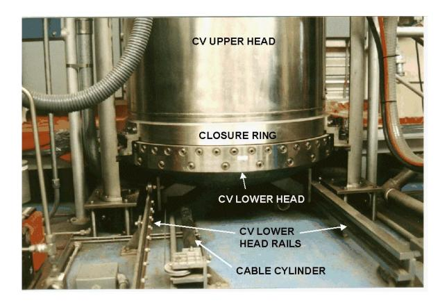
Figure 1-10. Drum Venting System in the Closed Position
