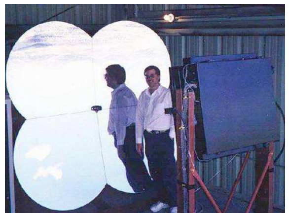
Figure 2.2: A single detector: a mirror and array of photomultiplier tubes.
