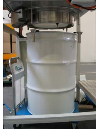
Drum Under Glovebox Fig. O
