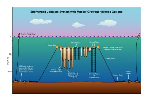
**Figure 8**: Drawing of an open-ocean blue mussel longline growout harness.
