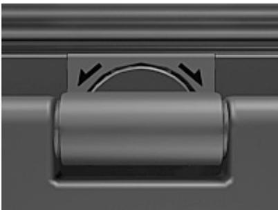
2. Unlatch the display latch and open the display by at least 45 degrees, preferably by 90 degrees.
