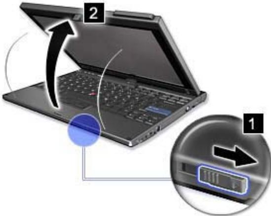
2. Open the display by at least 45 degrees, preferably by 90 degrees. Grasp the center of one side of the computer display with one hand while holding the keyboard bezel with the other hand; then rotate the display slowly clockwise or counter-clockwise (the figure below shows clockwise rotation as an example) until the back of the display is facing the keyboard. Your computer is now in the **picture frame mode**.
