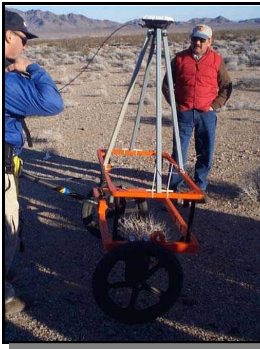
Fig. 2. Apparatus for sensing buried UXO. Its design positions the lower rectangle half a meter above the ground. The entire mass is about 31 kg as arranged for Camp Ibis.
