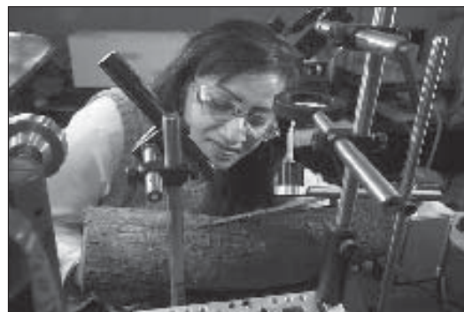
Madhavi Martin subjects a chunk of wood to laser-induced breakdown spectroscopy.
