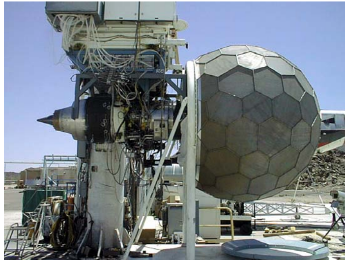
TFE731-60 Engine with Inflow Control Device (ICD)
