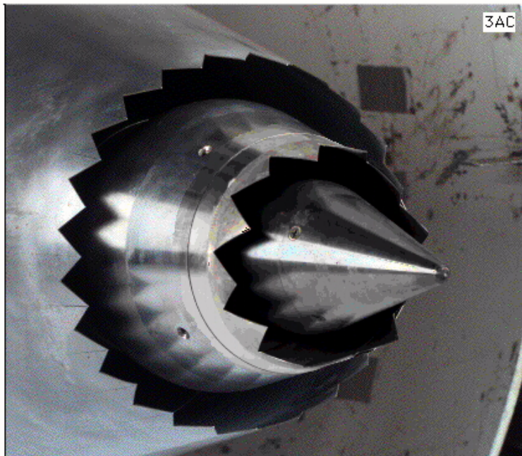
Fan Chevrons with Core Alternating Chevrons
