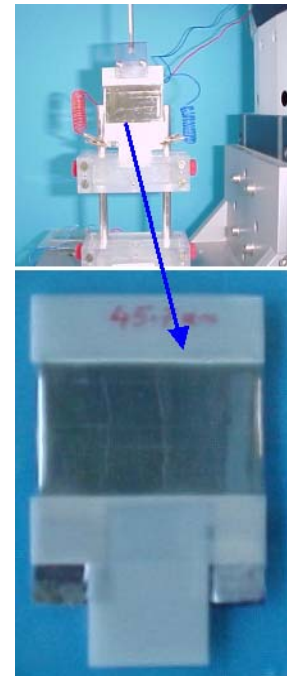
FIGURE 6: Silicone actuator of dimension 20x40mm and thickness 40 μm mounted on the electromechanical test bench. Strain at constant load is measured as a function of applied voltage.
