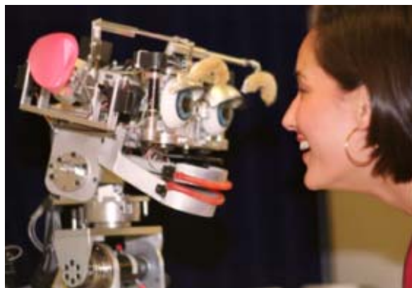
FIGURE 2: The Keynote Speaker, Cynthia Breazeal, MIT, with her Kismet robot responding to her expressions (courtesy of MIT Press Office) [ http://www.ai.mit.edu/people/cynthia/cynthia.html ].
