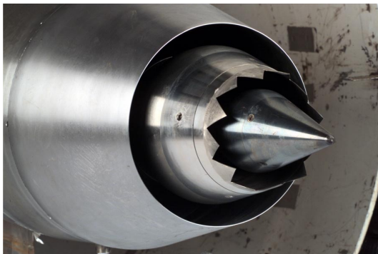
Figure 11. Separate flow nozzle with alternating chevron core nozzle (3A 12 B).
