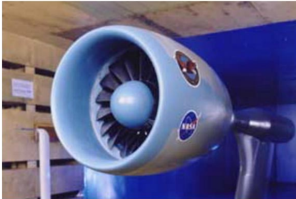
Figure 1. The Advanced Ducted Propulsor 22" scale model fan shown installed in the NASA 9'x15' wind tunnel.
