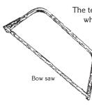
The teeth are needle sharp, so wear gloves when sawing and keep your hands clear of the cut and the blade. Carry bow saws by your side with the blade pointed down. Cover the blade with plastic blade guards or small diameter fire hose secured with Velcro fasteners. Always carry spare parts and plenty of replacement blades.
