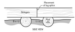
Figure 49—When using logs, notch the mudsill—not the stringer. Do not notch them more than one third of their diameter.
