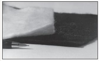
Figure 33—Felt-like geotextiles are easier to work with than heat-bonded, slitfilm, or woven products that have a slick texture.
