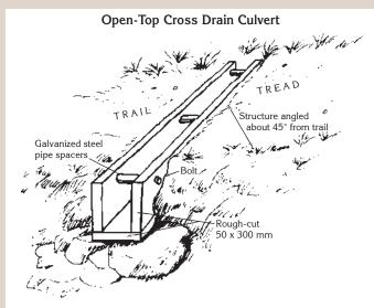
Figure 27—Open-top cross drains or culverts are not often chosen because they are a hazard to livestock, hikers, and bikers.
