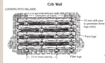
Figure 62—The characteristics of a crib wall. Treated logs are recommended (continued on next page).
