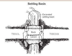
Figure 32-Settling basins help prevent culvert clogging.
