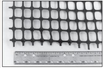
Figure 37—Geogrids are normally placed on top of a layer of geotextile to obtain separation from saturated soils.
