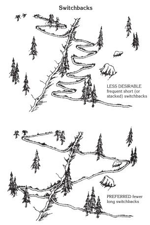
Figure 58—Long sections of trail between switchbacks are usually better than short—fewer switchbacks will be needed, with fewer turns to shortcut.
