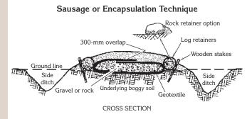
Figure 42-Sausage or encapsulation method.
