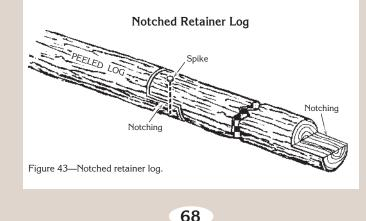
Anchor the logs with stakes or, better yet, large rocks along the outside. Inside, the fill and surfacing hold the retainer logs (Figure 44).
