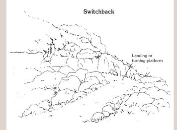
Figure 60—Switchback with a radial turning platform.
