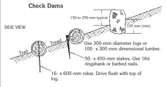
Figure 74—Check dams or retainer bars allow soil to rebuild on eroded trails (continued on next page).
