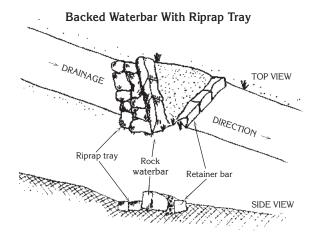
Figure 20-Reinforced or armored waterbars.
