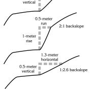
Figure 13—Slopes are noted in metric as a ratio of vertical to horizontal, or "rise" to "run."
