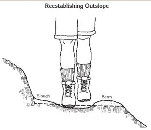
Figure 17—Remove the slough and berm, leaving the trail outsloped so water will run off. One fist's worth of drop for the length of a Pulaski is a good rule of thumb.
