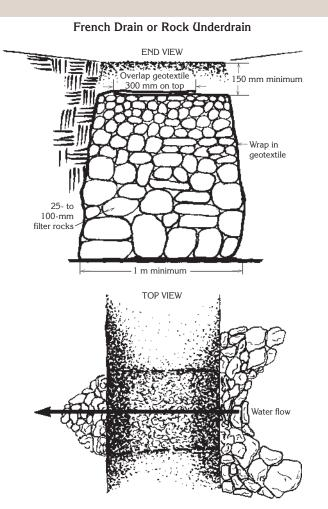
Figure 29—Wrapping French drains with geotextile helps prevent clogging. These are used to drain low-flow springs and seeps.
