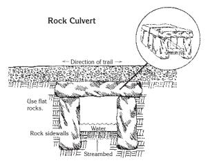
Figure 31—Rock culverts may also have stones laid along the bottom of the culvert. The perfect rocks shown here are seldom found in nature, except reportedly in Southwestern sandstone.
