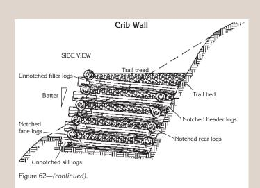
Rock or crib retaining walls are used when a sturdy wall is needed to contain compacted fill or to hold an excavation wall in place. Rock retaining walls are also called "dry masonry" because no mortar is used between stones. Rock, when available on site, is preferred over logs.
