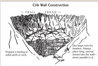
Figure 63—Rock placement and batter is critical on the first courses.
