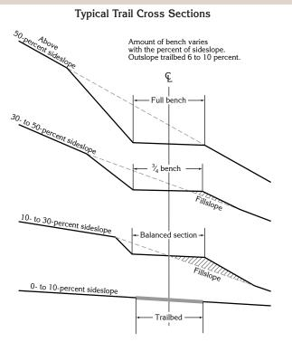
Figure 10—Typical trailway cross sections. Full-bench construction will give you the fewest problems—especially on steep slopes.
