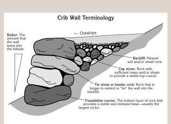
Figure 64—Terms used to describe crib walls.
