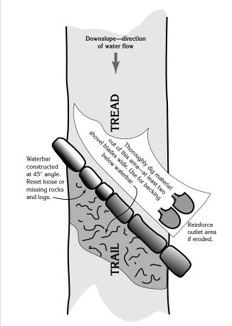
Figure 24—The key to waterbar maintenance is to ensure that sediment will not clog the drain before the next scheduled maintenance. Embed the rocks or logs a little deeper, cover them with soil, and you have a reinforced grade dip.
