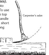
A square-tapered eye and handle end allows the head to tighten when swung, but also allows its removal for carrying and sharpening. Some adzes may have a small set screw to further secure handles to heads. An adze needs to be razor sharp to work. Never use this tool for grubbing.
