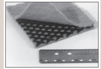
Figure 34—The net-like core of geonet allows drainage.
