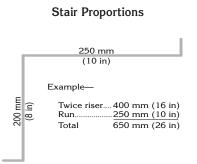
Figure 67—A general rule of thumb for stairs: Twice the riser plus the tread should equal 635 to 686 mm (25 to 27 in).
