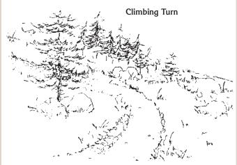
Figure 59—Climbing turns continue the climb through the turn. They can be insloped or outsloped.
