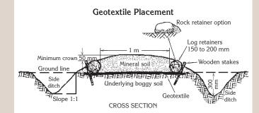
Figure 41—Place geotextile under the retainer logs or rocks before staking.
