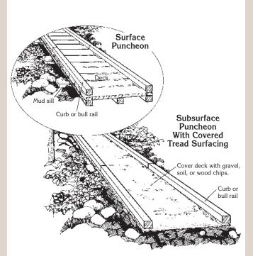
Figure 52—Subsurface puncheon with covered tread surfacing.
