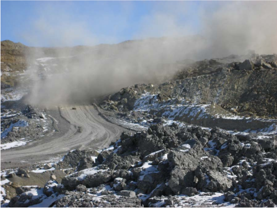
Figure 15 – Blast Fired with Austin E*Star Electronic Detonator Blasting System
