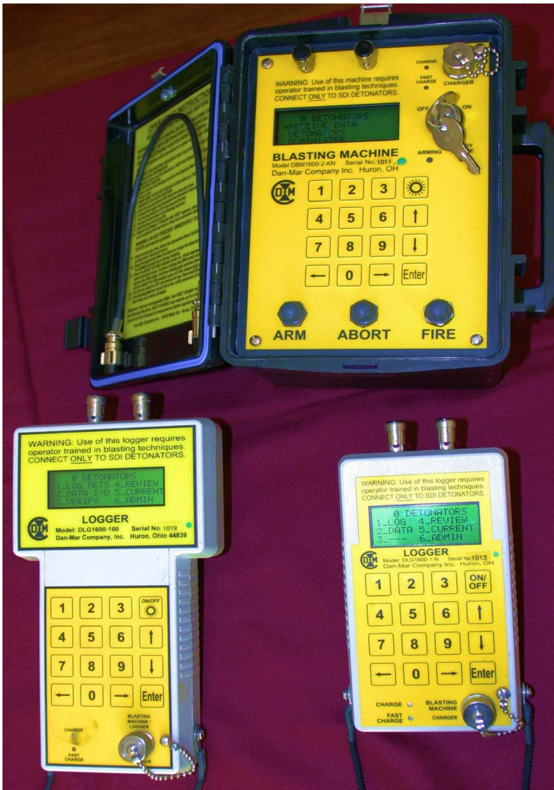
Figure 4 – Austin E*Star Electronic Detonator Blasting System
