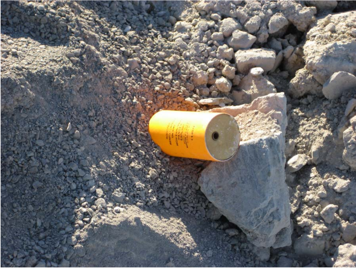
Figure 11 – Booster Placed at a Blast Hole
