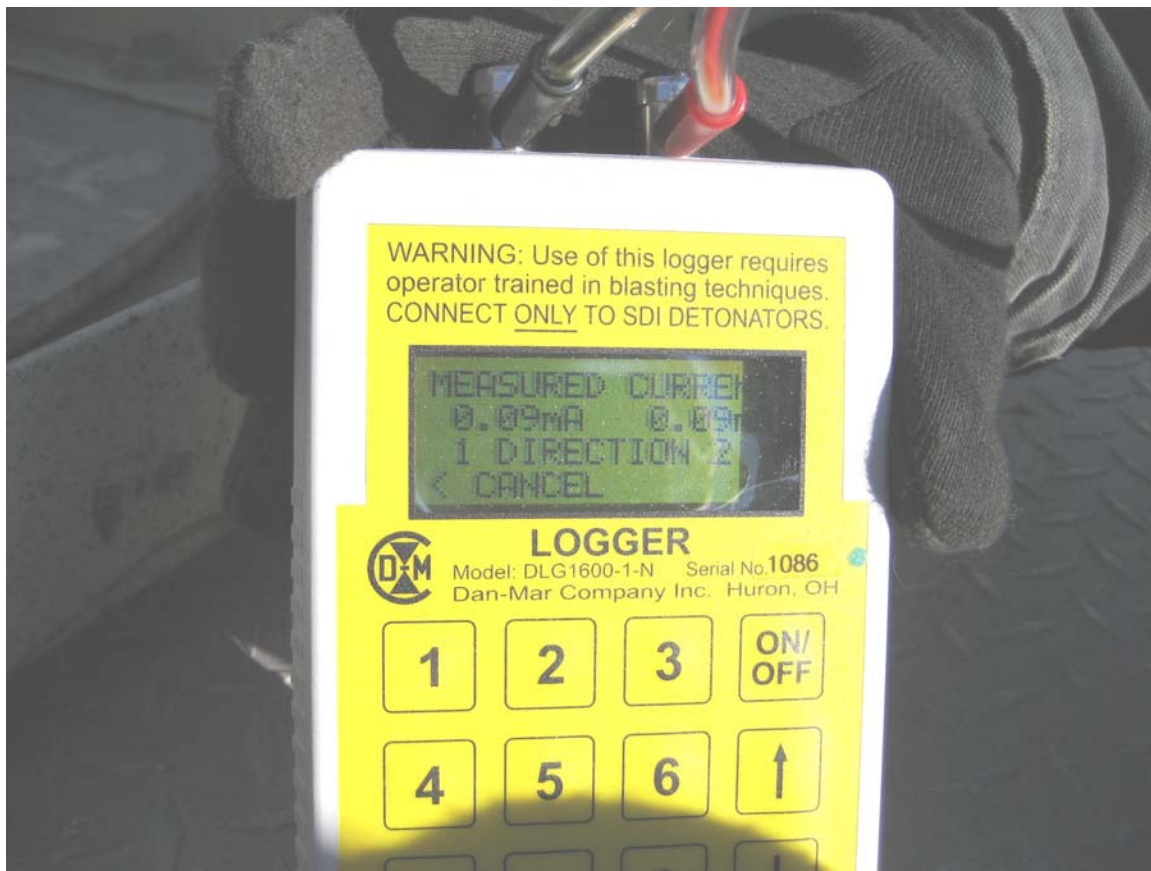
Figure 7 – Current Test of an E*Star Electronic Detonator using the Dash 1 Logger
