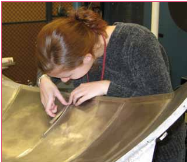
Graduate student Laura Berzak prepares to install magnetic pickup coils on the plasma-facing surface of the internal shell.
