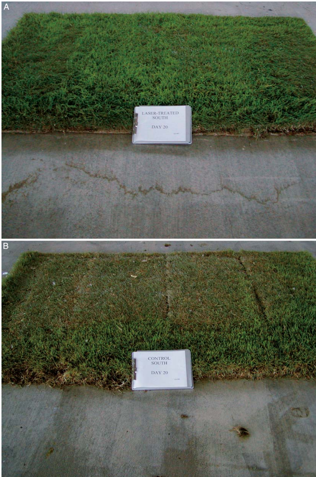
Figure 3. Grass sod from a laser-hazed (A) and control (B) subplot subsequent to the 20-day habituation test of a laser hazing system for repelling Canada geese.
