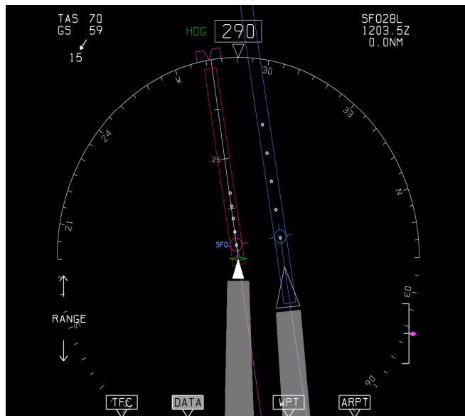
Figure 11. Heavy RIA/Heavy Conventional Approaching Touchdown with Complete Wake Protection for a Right Crosswind
