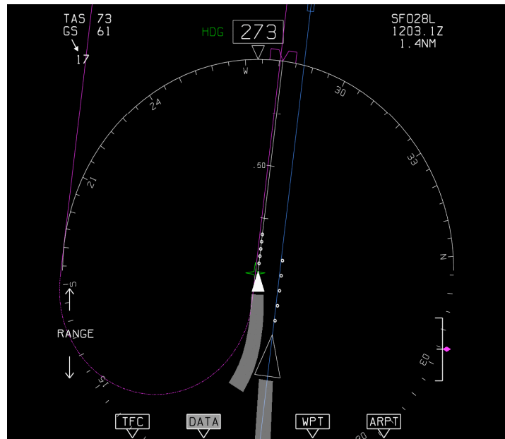
Figure 13. Heavy RIA/Conventional at Start of CSPA with a 10 KT Left Crosswind
