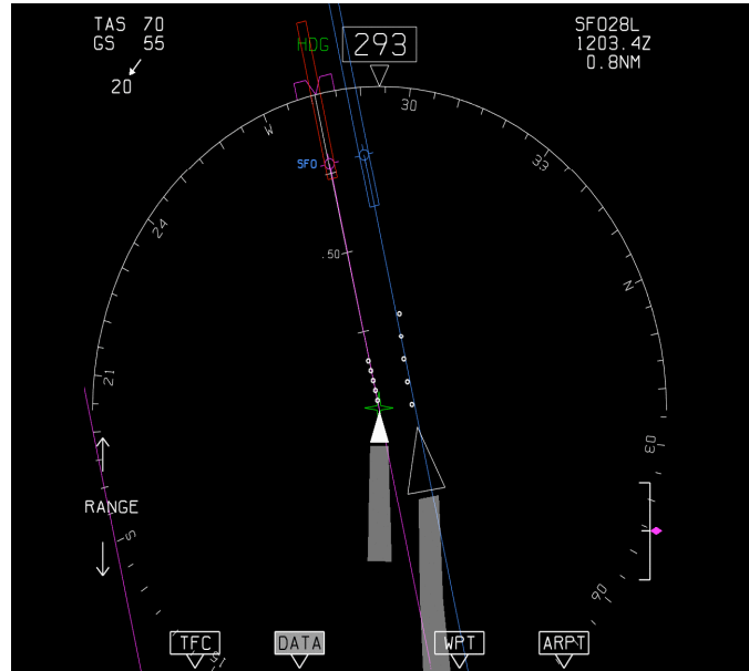
Figure 17. Heavy RIA/Conventional Approaching with a 15 KT (versus 10 KT Predicted) Right Crosswind - 0.8 NM on Final
