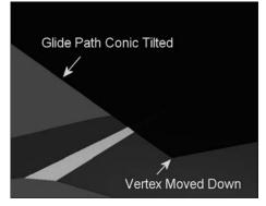
These two effects work in opposing directions. The tilting of the conic increases the height of the approach path, but the vertical moving down of the vertex decreases the height of the approach path.
