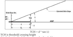
d is the longitudinal distance from the threshold to the point on the runway abeam the glide path facility  $\theta$  is the glide path angle
