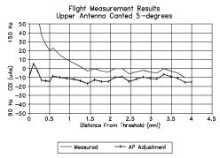
Figure 9: Paya Lebar Glidepath Approach after 5 degree Upper Antenna Rotation
