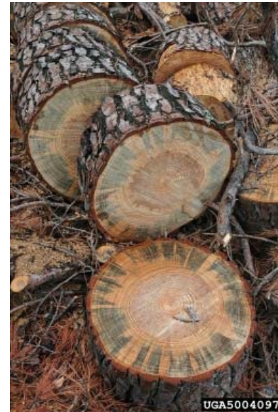
Fig. 39. Cross-section of Pinus taeda with wedge-shaped bluestain caused by Ophiostoma ips . Leptographium truncatum has a similar effect. Image from R.F. Billings, http://www.bugwood.org
