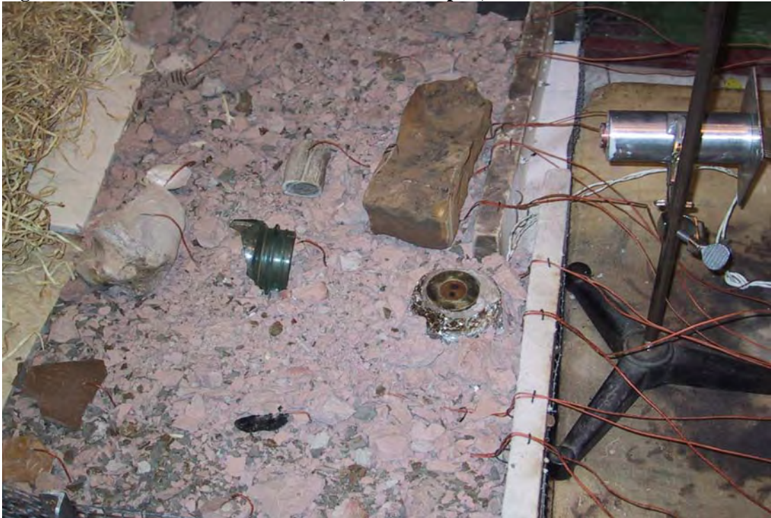
Figure 4.3: Sediment bed with artifacts, thermocouples, and radiometers.
