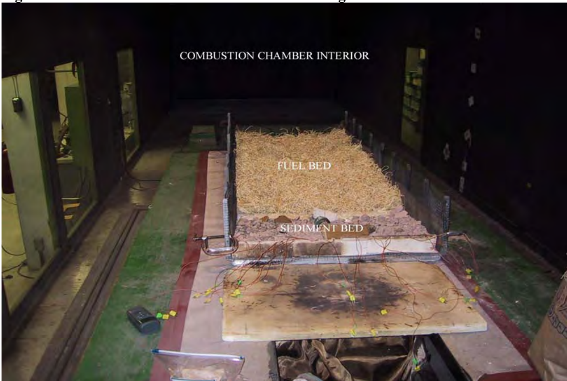
Figure 4.2: Interior of Combustion Chamber showing burn table.
