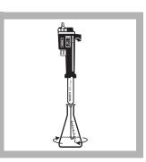
**6.** If the solution turns pink, titrate to a colorless end point. Place the delivery tube tip into the solution and swirl the flask while titrating with sulfuric acid. Record the number of digits required.
