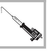
**3.** Turn the delivery knob to eject a few drops of titrant. Reset the counter to zero and wipe the tip.
