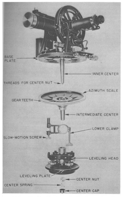
Figure 6-1b. Theodolite of the type used at land stations.
