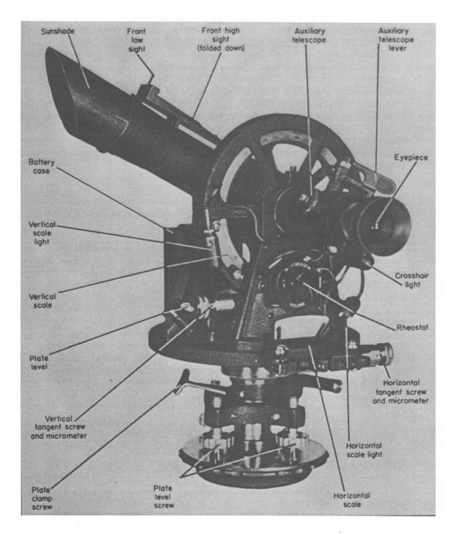
Figure 6-1a. Theodolite of the type used at land stations.
