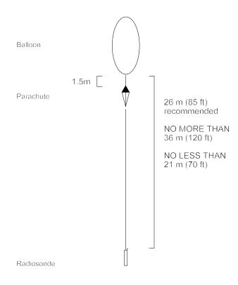
Figure 2-1. Schematic of a sonde with balloon, parachute, and train.
