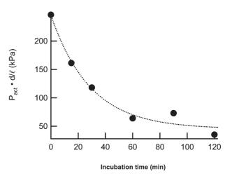
Fig. 4 Actuation pressure as a function of incubation time with fluoroalkyl coating. Substrate: fused silica capillaries. Polymer formulation: 5:5:3:3 ratio of TF-BDDA, 7FBA, 3FEA, and FC-84; photoinitiated with 10 mg ml<sup>-1</sup> of AIBN. Dashed line is exponential fit to data.
