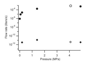
Fig. 7 Reverse flow rates through a microchip check valve can be reduced by a factor of  $2 \times 10^8$  as compared to forward flow rate. Circles: forward flow rate. Diamonds: leak rate backwards through closed valve. Valve geometry shown in Fig. 1. Working fluid: water (filled symbols) or acetonitrile (open symbols). Polymer composition: 2:1 w/w PE3: 1-propanol photoinitiated by 10 mg ml<sup>-1</sup> AIBN.
