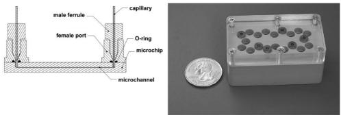
Fig. 2 High-pressure fluidic connections. (a) Male ferrule and capillary. (b) Female ports bonded to glass wafer. (c) Side cross-sectional schematic of bonded fittings and seals. (d) Alignment jig for attaching permanent epoxied fitting with O-ring seal.
