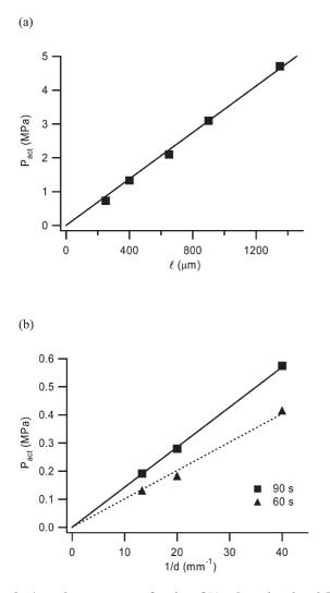
**Fig. 3** Actuation pressure as a function of (a) polymer length and (b) diameter. Polymer formulation: 3 : 3 : 4 ratio of 1,3-butanediol diacrylate, 3FEA, and 1-propanol. (a): 75  $\mu$ m diameter polymer elements in untreated fused silica capillaries. (b) 100  $\mu$ m long polymer elements in untreated silica capillaries at two exposure times.
