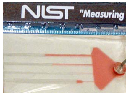
Figure 2. Milli-fluidics chip viscometer.
