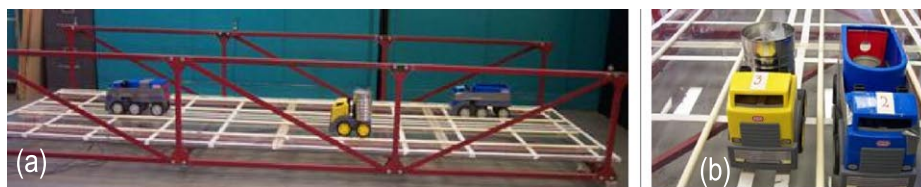
Figure 1: Experimental investigation of a model bridge (a) Bridge configuration with three traffic lanes (b) Model trucks used to model bridge dynamic response
