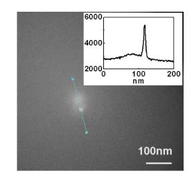
FIG. 5. (Color online) TEM micrograph for the 3  $\mu$ m long CNT section under  $0^{\circ}$  recorded with the electron beam underfocused by 2  $\mu$ m. Downloaded 05 Sep 2007 to 128.3.132.212. Redistribution subject to AIP license or copyright, see http://apl.aip.org/apl/copyright.jsp
