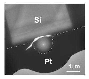
FIG. 2. Low magnification TEM micrographs of an isolated CNT section with a channel length of 0.72  $\mu$ m on a silicon substrate and with Pt deposit.
