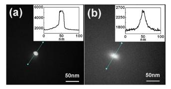
FIG. 4. (Color online) TEM micrographs of a 3  $\mu$ m long CNT section under a tilt of  $0^{\circ}$  (a) and under a tilt of  $1^{\circ}$  (b). The inserts show the intensity profiles of the transmitted electron beam in the imaging plane along the indicated line scans.
