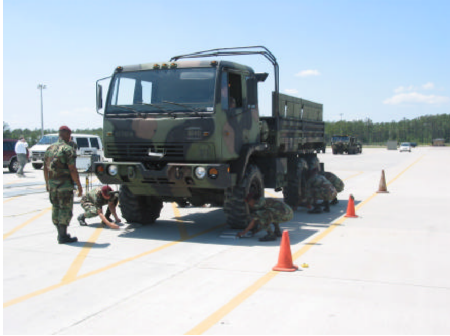
Figure 3 Positioning Portable Weigh Scale under Front of Wheels 3
