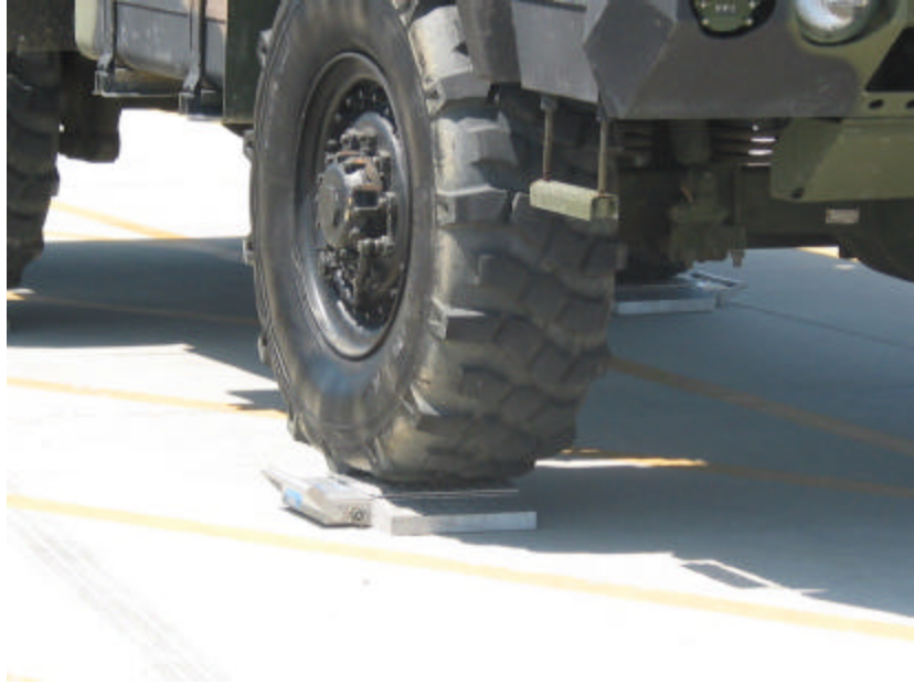
Figure 5 Close Up of One Axle on Portable Weigh Scale 5
