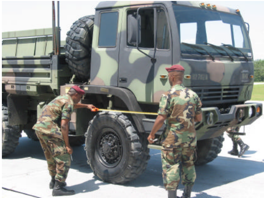
Figure 7 Measurement of Front of Vehicle to 1 st Axle on Static Scale 7
