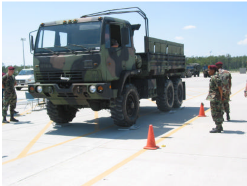
Figure 4 Weighing Vehicles on Portable Weigh Scale 4
