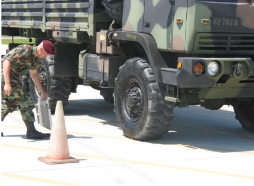
Figure 2 Preparing to Position Portable Weigh Scale 2
