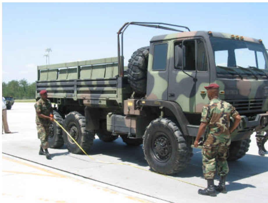
Figure 8 Measurement of Front of Vehicle to 2 nd Axle on Static Scale 8
