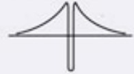
Fig 1b: schematic charge distributions of the vacuum electrons in the neighbourhood of an electron
