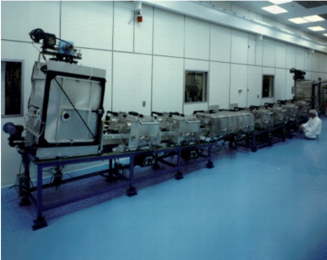
Figure 30. Double-junction roll-to-roll plasma-CVD processor, previously used as United Solar's production machine. This machine will be used as an experimental machine for much of the work proposed in Tasks 1 and 4.
