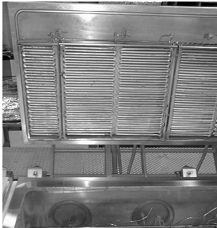
Figure 6. Ribbon heater assembly detail.
