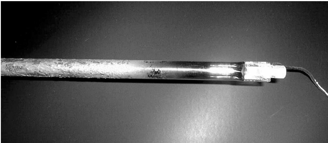
Figure 1. Photograph of a quartz IR heating lamp from the 5 MW production machine.
