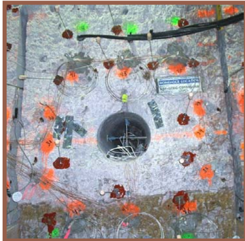
In Situ Slot Compression Testing
