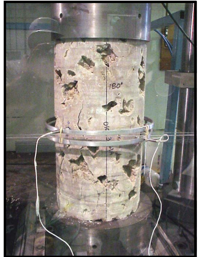
Laboratory Testing of 12-inch Cores
