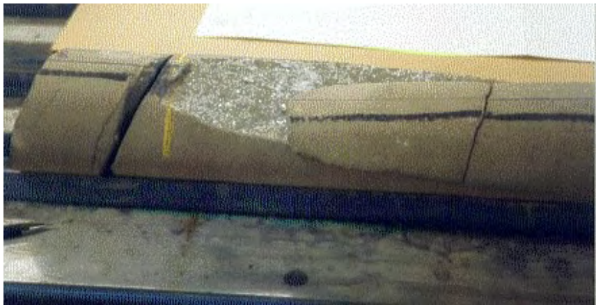
Concave downward parabola formed as the main cored fracture exits the core near 17,818' MD. Euhedral calcite crystals visible as bright specs on fracture face.
