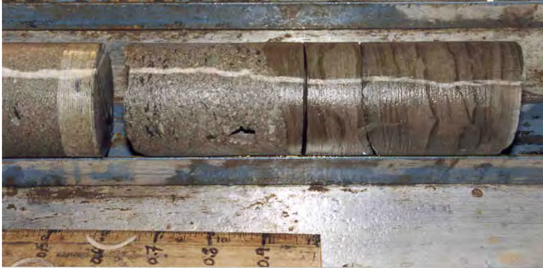
The fracture at 13, 712' cuts across lithologic boundary between pebble conglomerate and sandstone. The lower end of the fracture was not observed. Up is to the left.
