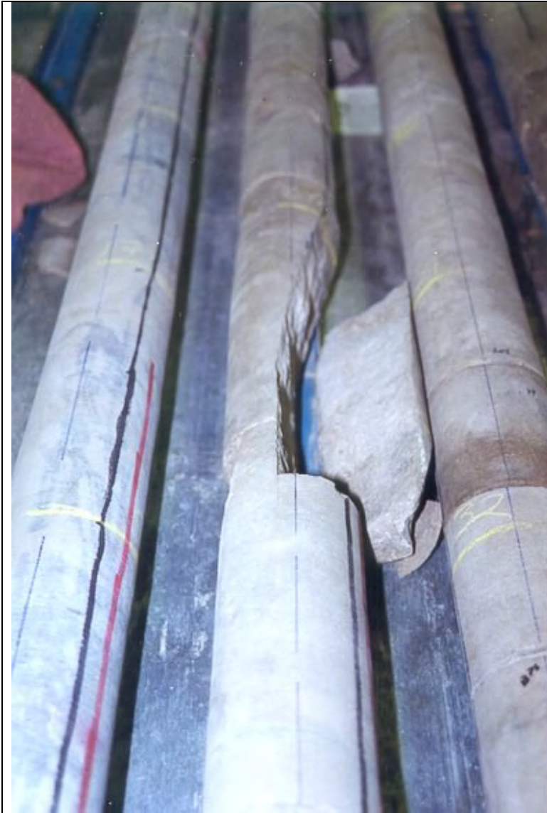
Fig. A-6. Coring induced petal fracture at 17,818' MD
