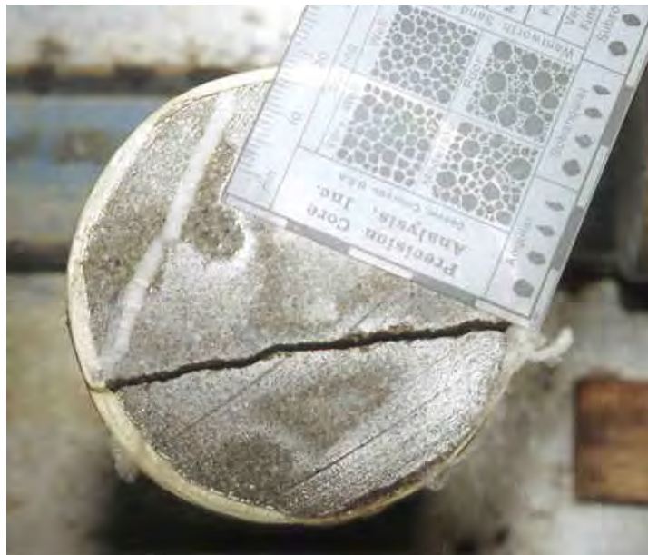
The healed, calcite-filled natural fracture is the white line to the left center of the photo parallel to the scale edge of the grain size comparator. The jagged black line running left to right is the trace of a drilling induced petal fracture. The angle between the fractures was measured to be 60 degrees. The data supports a rotation of the stress field between the time of the natural fracture and the collection of the core. View is looking up the core.
