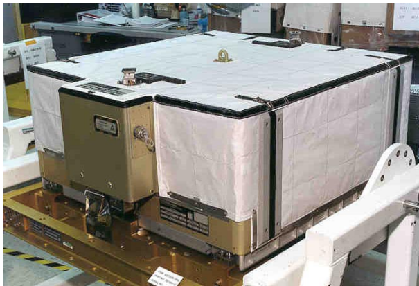
FIGURE 2. ISS BATTERY SUBASSEMBLY ORU WITH MLI BLANKET
