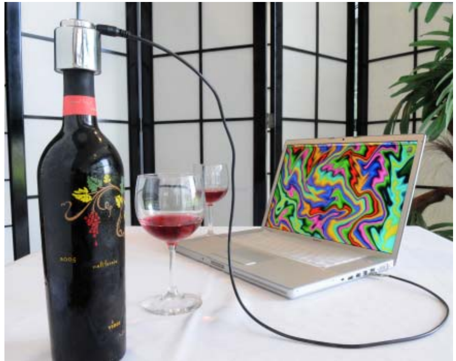
A new cap invented by Argonne’s Vulnerability Assessment Team can detect fraudulent or tampered wine. By plugging the cap into a computer through a USB cable, a wine buyer or auctioneer can determine if the wine inside is genuine. New generations of the cap will contain a color sensor that detects a particular tiny section of a tie-dye pattern located under the cap.
