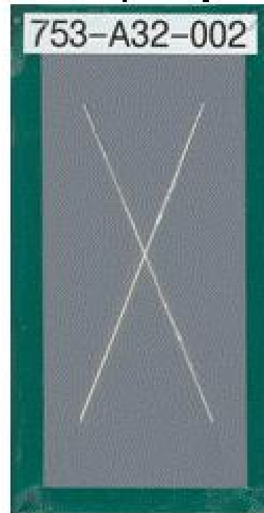
BAM-PPV in Oxsel-100 Non-Chromated Deft 02-GN-083 MIL-PRF-85285
