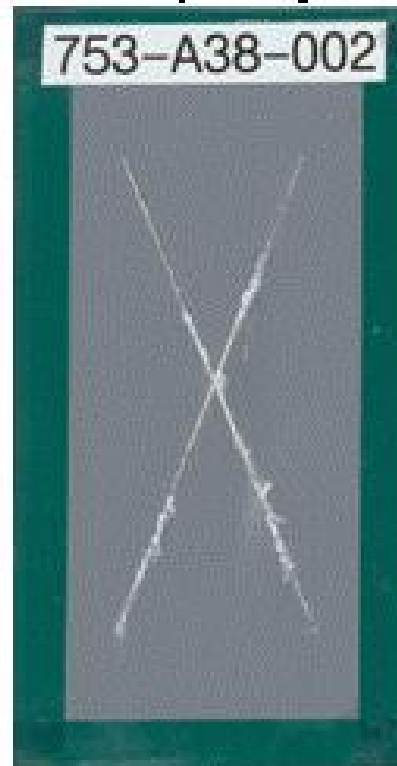
BAM-PPV in Oxsol-100 Non-Chromated Hentzen MIL-PRF-85285
