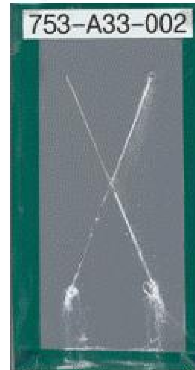
BAM-PPV in Oxsel-100 Non-Chromated Deft 02-GN-083 MIL-PRF-85285 APC
