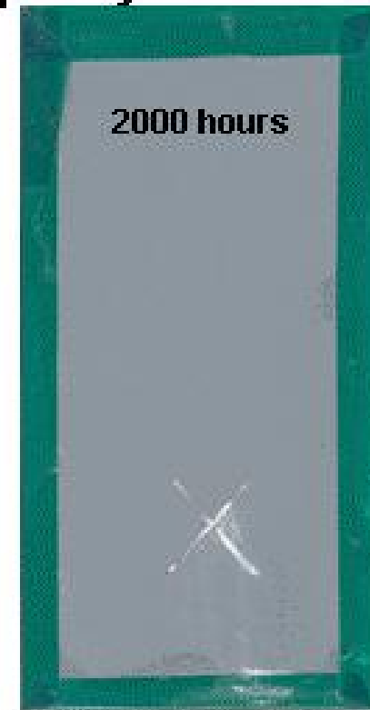
MEH-PPV in Oxsol-100 + MIL-PRF-23377 + MIL-PRF-85285 APC
