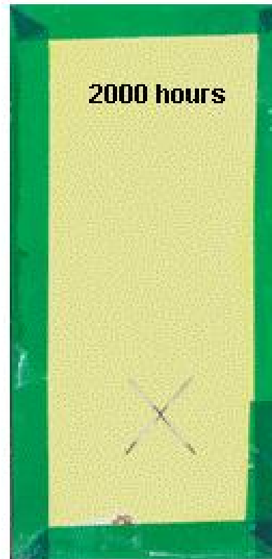
MEH-PPV in Oxsol-100 + MIL-PRF-23377
