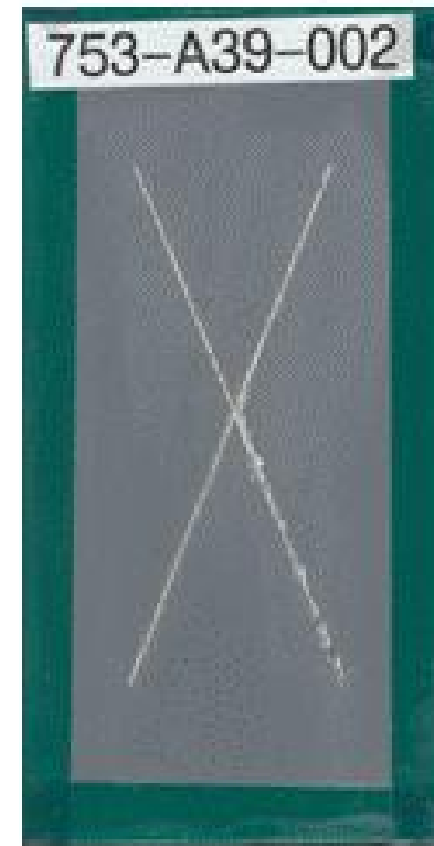
BAM-PPV in Oxsol-100 Non-Chromated Hentzen MIL-PRF-85285 APC
