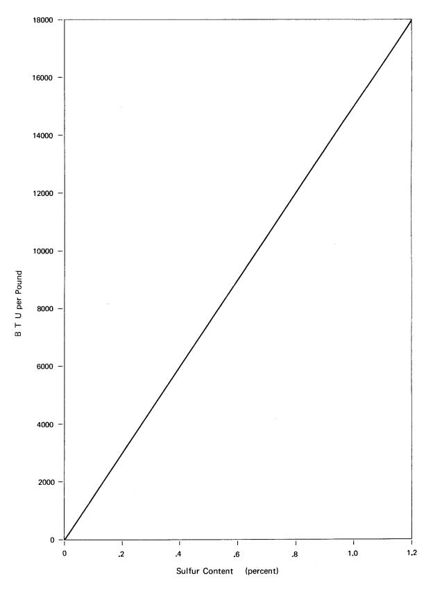
**Figure 8.** Maximum sulfur content that will meet EPA standard of 1.2 pounds SO<sub>2</sub> per million Btu (assume 10 percent of sulfur remains in ash).
