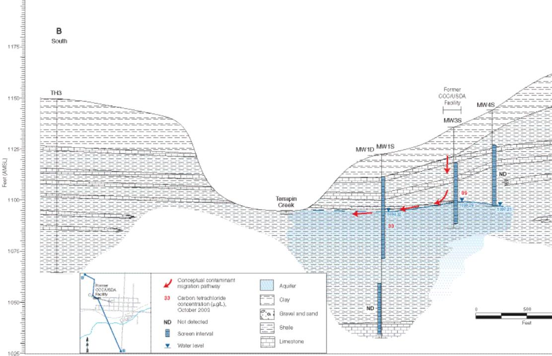
FIGURE 4.5 Inferred contaminant migration pathway at the former CCC/USDA facility at Morrill, displayed on interpretive geologic cross section B-B<sup>-</sup> (vertically exaggerated; Figure 3.8 in Argonne 2003).
