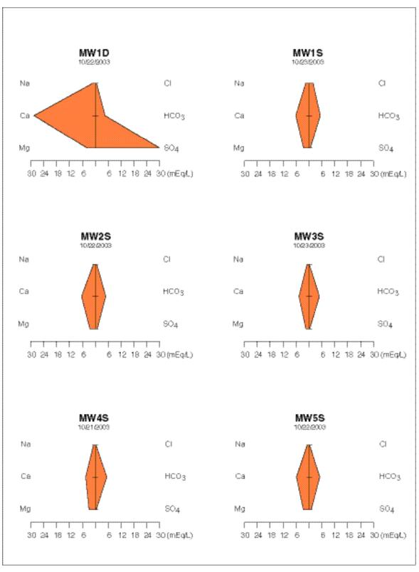
FIGURE 4.1 Major ion compositions (milliequivalents per liter) for groundwater samples collected at Morrill in October 2003, displayed as Stiff diagrams.
