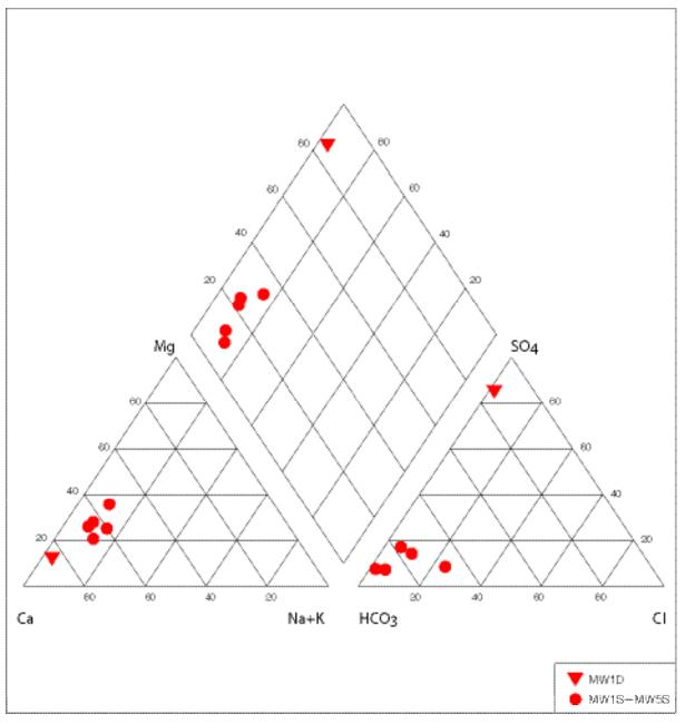
FIGURE 4.2 Major ion compositions (percent of total equivalents per liter) for groundwater samples collected at Morrill in October 2003, displayed as a Piper trilinear plot.
