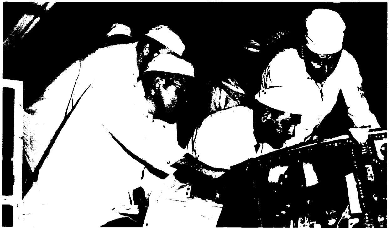
MSC-FLORIDA OPERATIONS Test Conductor George Page, Assistant Chief of Inspection and Quality Control Joe Bobik, and Inspector L. Dotson conduct final review of Gemini Spacecraft-2 cabin section prior to mating with RCS system.
