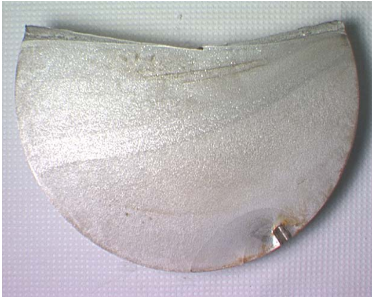
Fig. 35. Cross-section of cracked shaft.
