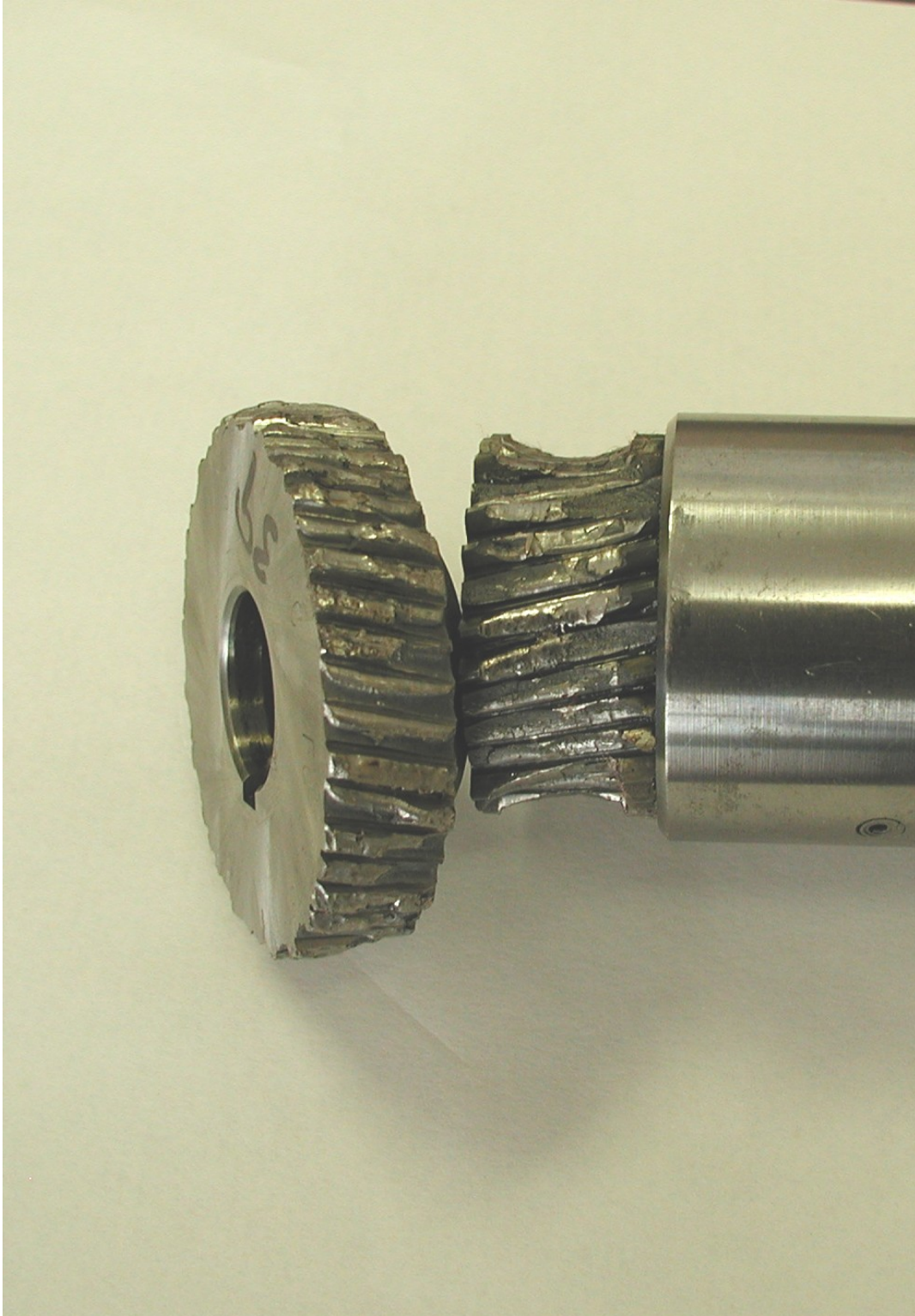
Fig. 25. End-of-life failure in PSU Run No. 39 (broken/rounded-off teeth on both the gear and pinion).
