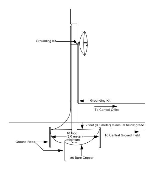
Figure B5: Building Mounted Installation
