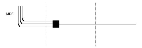
22-Gauge Polyethylene Insulated Conductors with PVC Covering
