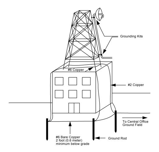
Figure B6: Tower Ground Kit Installation
