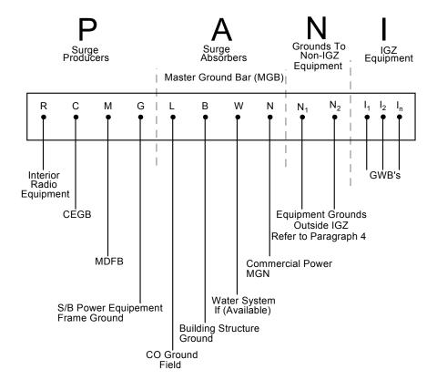
Figure 2: Outdoor Grounding Conductor Connections
