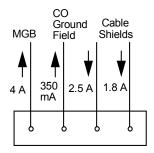
Figure C3: Undesirable Size Reduction in Grounding Conductor
