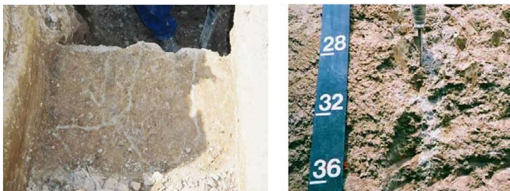
Figure 9.—At left, the top of the fragipan is exposed in an area of Ava silt loam, revealing very coarse prismatic structure outlined by light gray silt. At right is a side view of the profile; depth is shown in inches.
