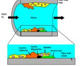
Over time, the iron surface is corroded and tubercles are formed
