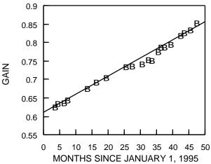
Fig. 3. GOES-8 VIS channel gain trend, where GAIN is in  $Wm^{-2}sr^{-1}\mu m^{-1}$ .
