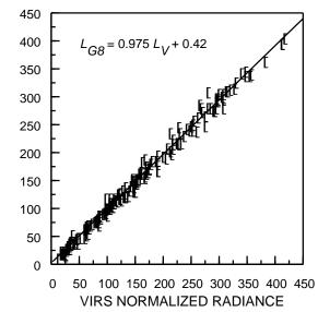
Fig. 4. Regression of VIRS and GOES-8 VIS channels for January 1998. Radiances given in  $Wm^{-2}sr^{-1}\mu m^{-1}$ . analysis.
