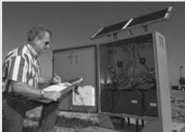
George Williams of Code FEF at an Ames test site where grounding electrodes are evaluated.
