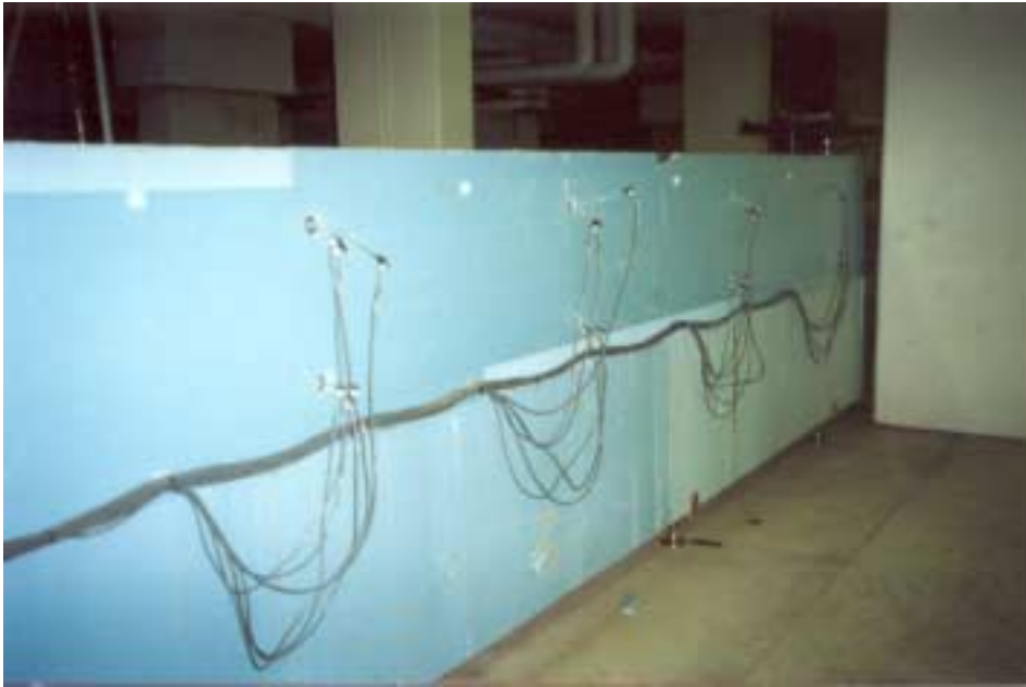
Figure 10. Photograph of test box with tensiometer tubes connected to pressure transducers exiting the side of the box.
