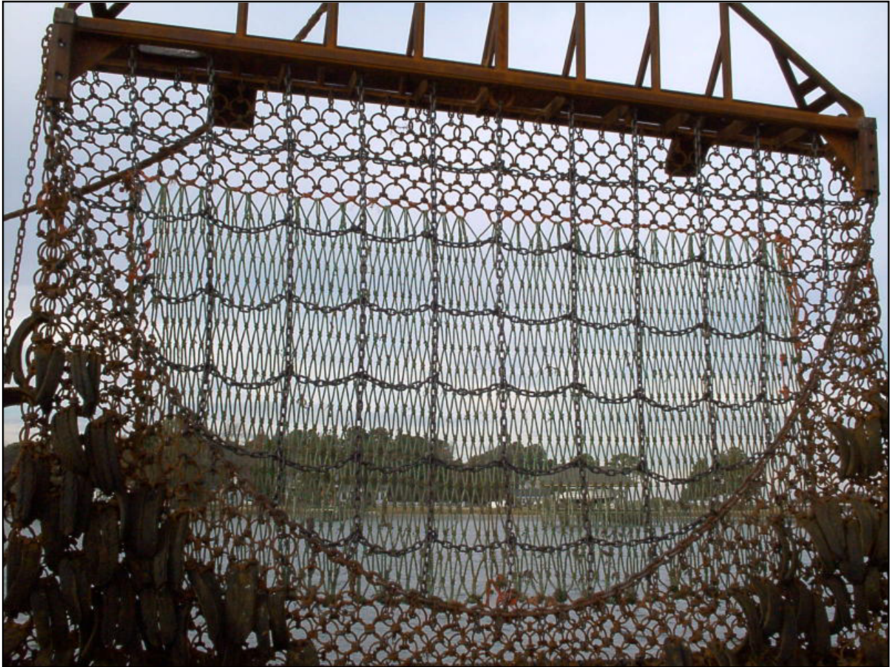
New Bedford-style scallop dredge rigged with turtle chain.
