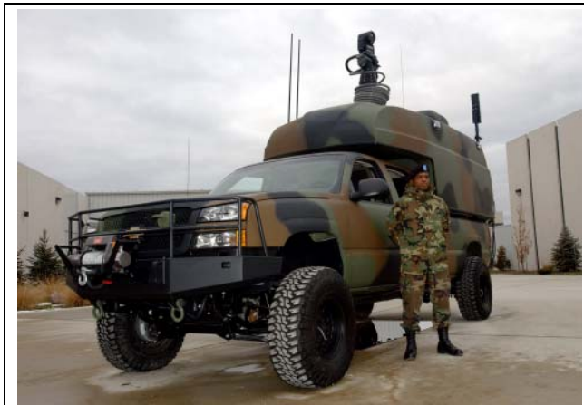
2003 Diesel Hybrid Electric Military Truck (w/fuel cell APU)
