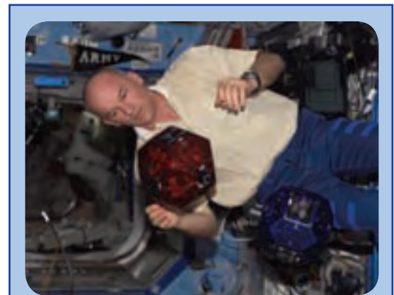
Astronaut Jeffrey Williams, Expedition 13 NASA science officer, checks the Beacon/Beacon Tester for the Synchronized Position Hold, Engage, Reorient, Experimental Satellites (SPHERES) on August 19, 2006. SPHERES, which uses robotic mini-satellites, tests the basics of formation flight and autonomous docking that should be useful in future multiple spacecraft formation flying. The first satellite arrived at the ISS by Progress spacecraft in April 2006, and STS-121 delivered the second, blue satellite. A third, yellow satellite will launch on STS-116. Although the SPHERES satellites have been tested on Earth, 2006 marks the first tests in space. (NASA)
