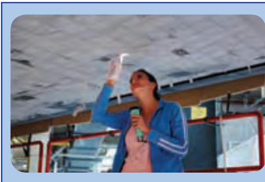
United Space Alliance technician Erin Schlichenmaier uses a flashlight to inspect tile repair on Discovery 's underside in November 2005. In preparation for STS-121, technicians replaced older Shuttle tiles around the main landing gear doors, external tank doors, and nose landing gear doors with a new type of tile called BRI-18. The new tiles are more impact resistant than previous designs. Technicians also developed a new procedure to ensure that gap fillers, which fill the tiny gaps between tiles, do not protrude and pose a hazard during the Shuttle's re-entry into Earth's atmosphere. During the STS-114 mission in 2005, a crewmember conducted a spacewalk to remove a protruding piece of gap filler spotted on Discovery 's underside. (NASA)
