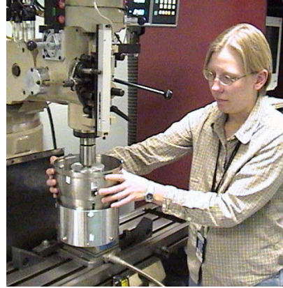
Figure 10: Diagram and Photograph of Friction Coefficient Measurement Rig
