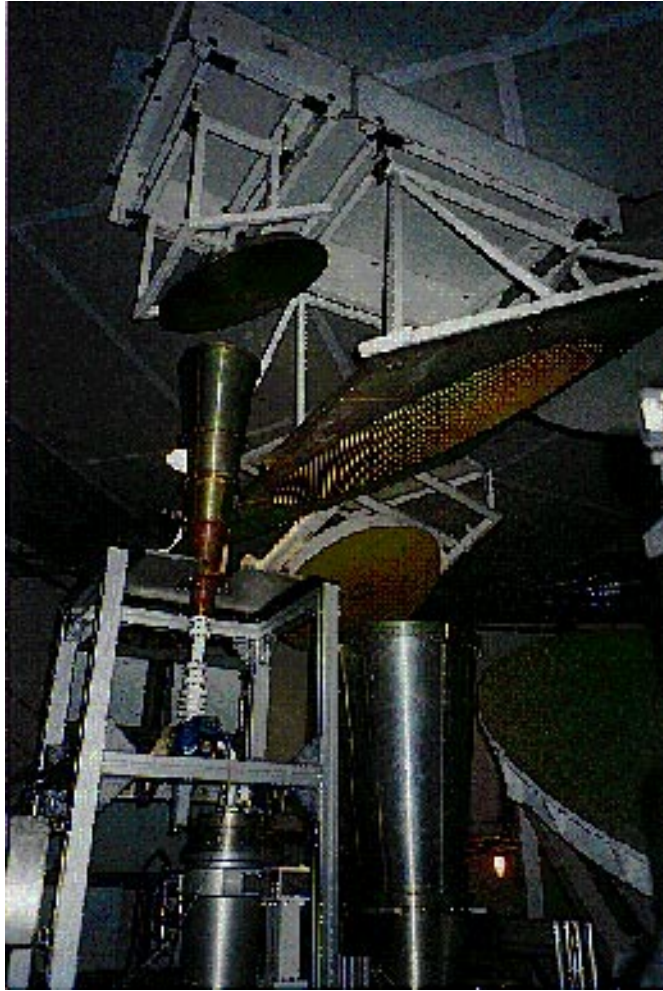
Fig. 12. Feed system installed in BWG antenna.
