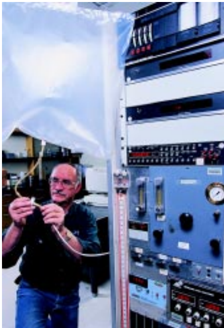
Technician Eldon Shetler readies an air sample bag for analysis of respiration gases collected during an indirect calorimetry study. Data on heat production will help the DECI model predict energy partitioning in growing cattle.
