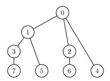
The figure is structured with time flowing downwards. That is, for a multicast operation expressed over a 2-nomial tree, task 0 sends a message to task 1 in the first time step. Then, task 0 sends to task 2 while task 1 sends to task 3. In the final step, task 0 sends to task 4, task 1 sends to task 5, task 2 sends to task 6, and task 3 sends to task 7—all concurrently. The following expressions also hold, assuming there are a total of eight tasks in the computation:
